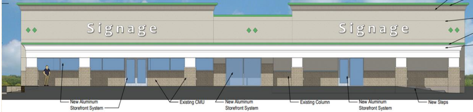
② Renovated Main St. Elevation 3/16" = 1'-0"
